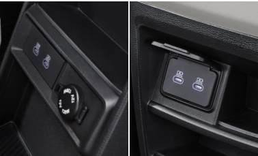
USB Type-C Ports (Front: 1 Charging, 1 Data & Charging / Rear: 2 Chargings)
