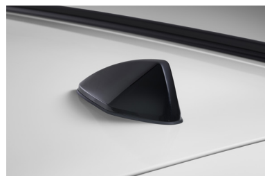
Shark-fin antenna with GLONASS, DAB and GSM
