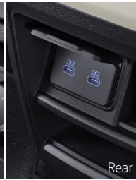
12V power sockets and 27W USB-C chargers in the front and rear
