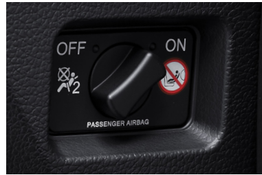
Passenger airbag on/off switch
