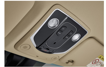
Overhead console with map lights (and sunroof control switch)
