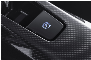
Electronic parking brake with auto-hold function
